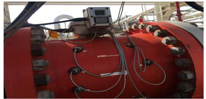
Fig.5 Experimental measurements for ATTF Ultrasonic meter
